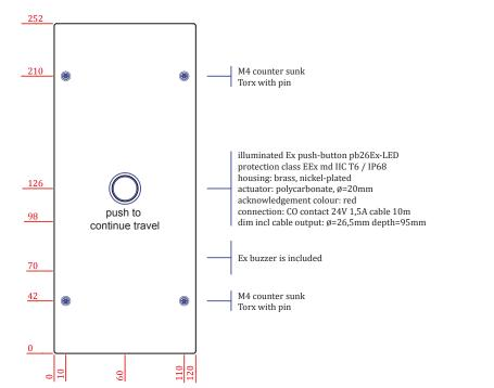
The optional Ex operating panel is used as an additional operating panel in the car. It includes an Ex indicator lamp "light grid interruption", an Ex buzzer and an Ex "continue" pushbutton. The cover plate consists of V2A, grain 240, includs engraving and M4 Torx screws with internal pin. The installation depth is 100 mm. An optional housing can also be supplied.
